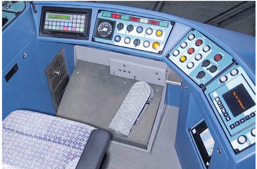
Dead Man's Pedal Switch TFS 001 installed below control panel
